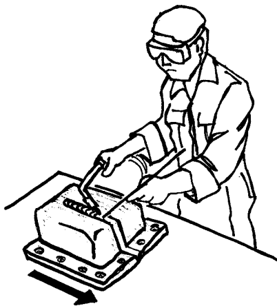
Leftward welding
