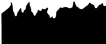
Structural peaks acting as attack points for corrosion
