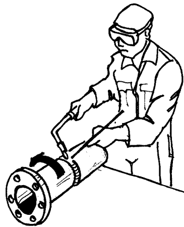
Rightward welding
