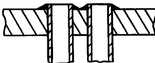
Boiler tubes welded to boiler tube plate
