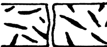
A crack in cast iron. The carbon flakes in the metal are saturated with oil.
