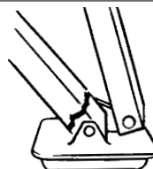
Steel that is difficult to weld, and steel subject to vibration and loads (engine foundations etc.).
