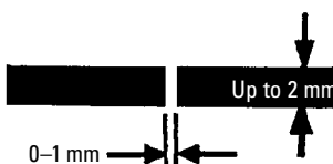
Close square butt joint
