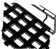
Grading and vibrating screens. Edges are welded with Abratech-330. Large surfaces filled in with Ceramigrade Abrashield
